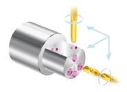
By using the Y-axis, the machining time for off-center drilling and off-center tapping can be shortened. The tapping accuracy with a rigid tap is also improved. (01RY)
