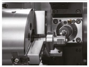
Combining an original double-column type Y-axis mechanism (01RY) with a turret slide on the Y-axis only instead of having X-axis and Z-axis slides enables high-precision machining in turning work.
