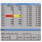
Used to set and reset the tool counter stop value and enter the tool wear offsets.
