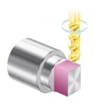
Accurate positioning by the C-axis and high precision combined machining by the Y-axis allow for a wider range of machining.(01RY)
