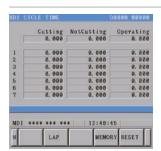
Measures the cutting time, noncutting time and running time in each cycle.
