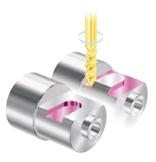
Separating the machining into rough cutting and finishing improves both the accuracy and the quality of the machined surface. (01RY)
