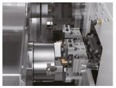
4. The spindle moves to the position of the IN hand and receives the blank from the IN hand.
